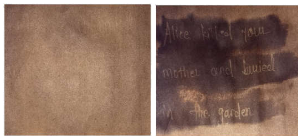
a) Sample writings after burning (not visible) b) After spraying with ammonia solution (visible)
