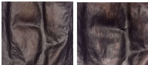
a) Sample writings after burning (not visible) b) After spraying with ammonia solution (very faintly visible).
